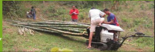
Rubber racked mini-crawler conversion
